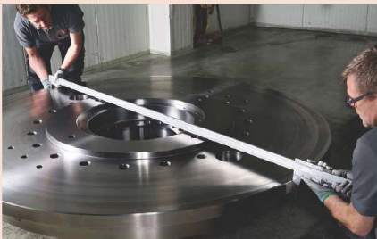
Radiused jaws for accurate ID measurement
